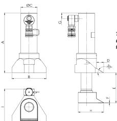
The swivel coupling is capable of rotating 360° even under pressure which guarantees highest possible flexibility when handling the tool.
