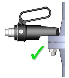
Place the tool on the nut with the flat surface of the cutting head flat against one of the nut flats and the Cutting Tip centered. Ensure the bottom face of the cutting head sits flat on the same surface that the nut is seated.
