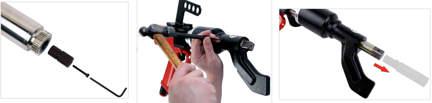
FIGURE 15 – Drive square replacement
