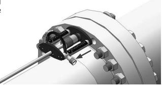
**20.** The Pull Rod complete with pull nut and washer can now be withdrawn from the flange joint.
