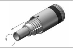
**8.** Having removed the collet assembly please note the centre dab marks indicating the position of the first collet section. Please also note that the collet segments are arranged on the cage such that the external ridges form one continuous thread.
